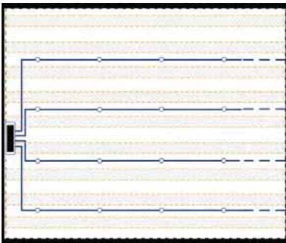
Figure 16 .- Sampling pipe layout for storage rack area, where racks stop well below the ceiling (non-branched pipes parallel to rack orientation)
