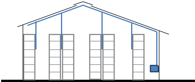
Figure 19. Example of drop-down pipes for in-rack ASD
